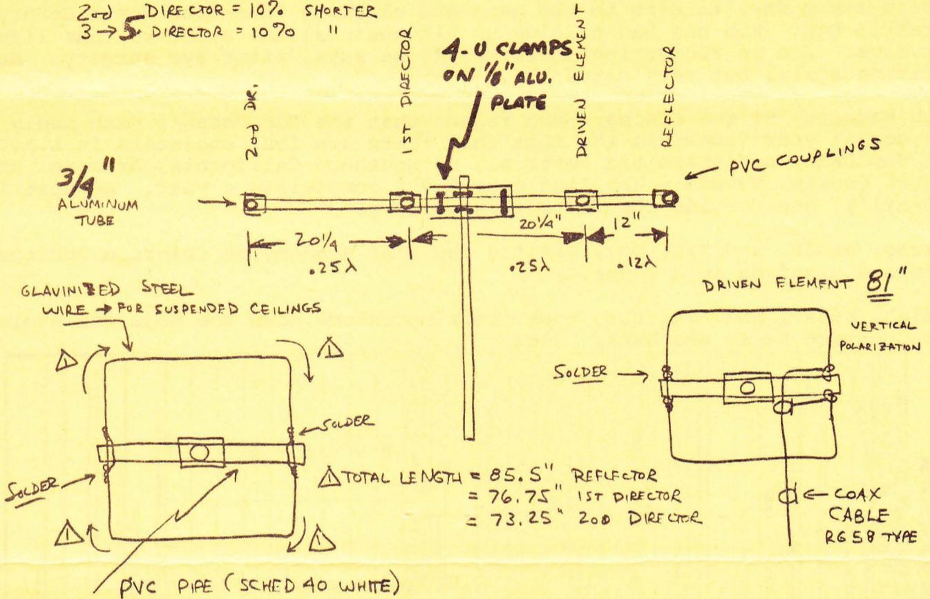
The antenna is made from 1/2" aluminum tubing and PVC pipe fittings. The elements are 1/8" galvanized steel wire of the type used to suspend ceilings, which is usually available at the larger building supply stores.
