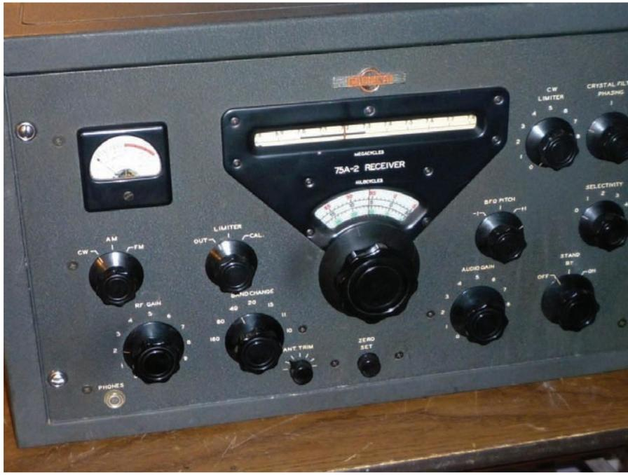
SSB, CW and AM, signals were handled very differently. AVC was only available for AM. On receivers of this era, when the BFO went on, the AVC went off!
